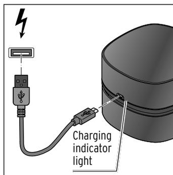
1. Connect the mini table vacuum cleaner to a USB mains adapter (not included) as illustrated using the micro-USB charging cable provided.
