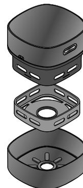
1. Hold the table vacuum cleaner over a rubbish bin and pull the collector tray down and off.
